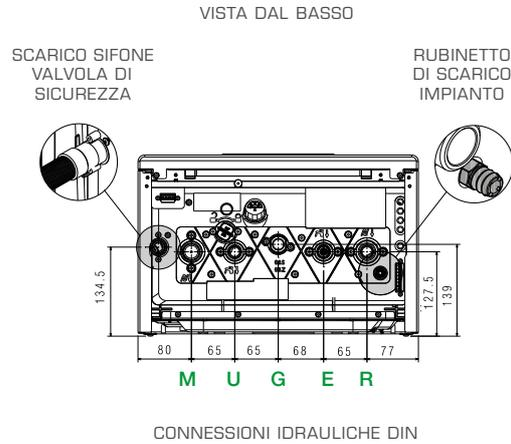
DISTANZA DEGLI ATTACCHI DAL MURO STUDIATA PER UNA FACILE SOSTITUZIONE, ANCHE SU SEQUENZA DI ATTACCHI DIVERSA
