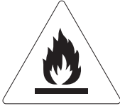
Caution: Risk of fire/flammable materials
